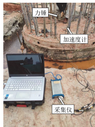
图6 实测桩顶动刚度试验现场 Fig.6 Test site of pile head dynamic stiffness
